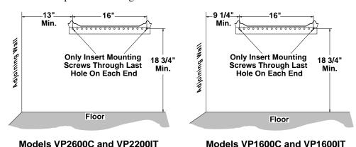
Figure 8 - Mounting Bracket Clearances
